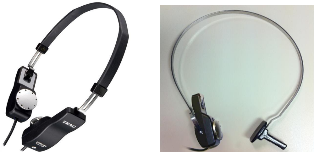
Figure 1: The bone-conduction transducer in its unmodified state (left) and after being adapted for audiometric use (right).
